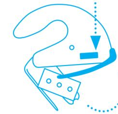
Press the catch again and insert the metal foot back into the handle until it **clicks**. Check that the foot is correctly inserted.
