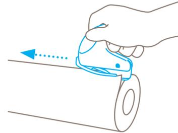
**Pierce** film and paper sheets at the required position using the point of the metal foot.
