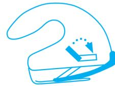
**Lift** the catch and move downwards until its end covers the blade change button.
