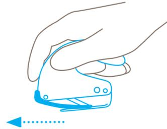
Cut by **pushing** and moving forwards.
