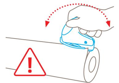
Only cut by sliding. Cutting by levering may break the metal foot.
