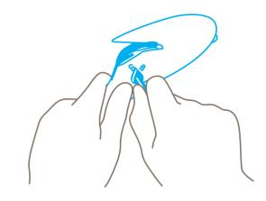
Use the locking key to lock the blade change mechanism ("lock closed").
