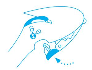
Finally, close the blade cover and push the blade holder **back into the handle**. With a click, everything is in place.
