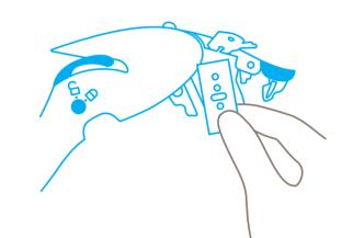
You can now lift up the blade cover to either rotate or change the blade.
