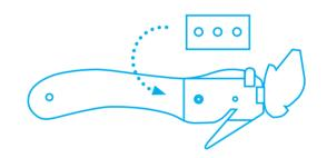
Re-insert the blade **exactly** over the locating lugs and thread.
