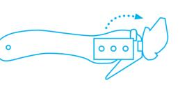
You can now lift up the blade cover and either reverse or replace the blade.
