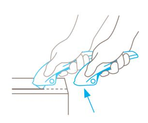
The blade automatically retracts into the handle the moment cutting ceases. Even when the lever is **still being squeezed.**
