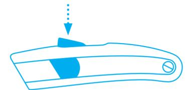
Now **rotate or change the blade** and carefully release hold of the slider. Close the rocking device.
