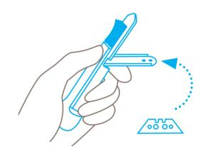
Use your index finger to slowly **fold out the blade holder downwards**. Use the other hand to remove the blade to either replace it or turn it around.
