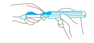
Use the slider to **push** the plastic insert back and out of the handle. Don't pull the insert while holding onto the slider.
