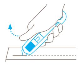
Always remove your **thumb from the slider** to For best results, cut plastic strapping band ensure automatic blade retraction.
