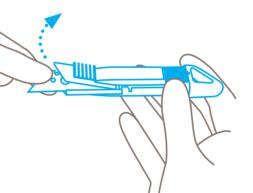
Take hold of the blade and nudge the blade cover open: either rotate or replace the
