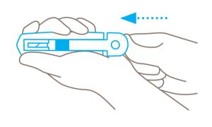
Make sure you position the blade **exactly** over the locating lugs, close the blade holder upwards. Attention: Never hold your hand in front of the blade exit!
