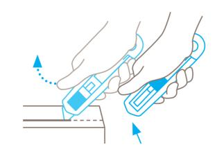
Following cutting, the blade immediately retracts into the handle. Condition: you have released hold of the slider.
