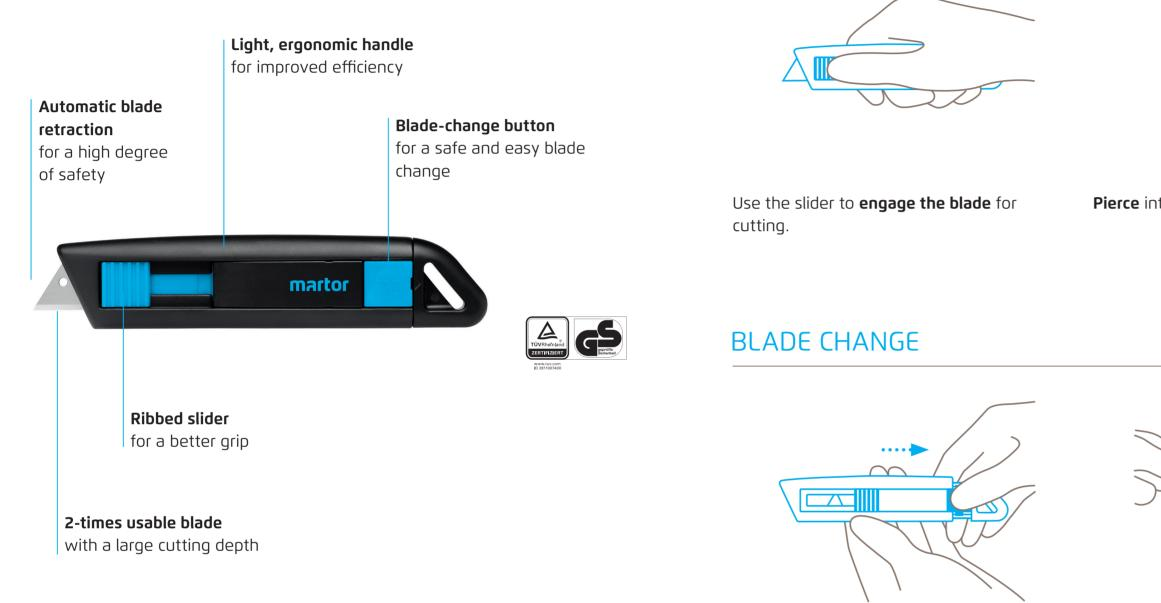
Press the blade-change button and **pull out** the plastic insert.
