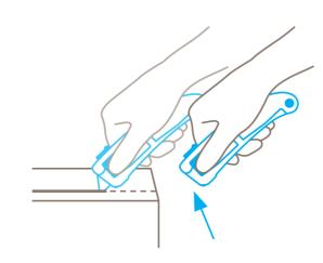
The blade automatically retracts into the handle the moment cutting ceases. Even when the slider is still **being held forwards**. Your SAFEBOX is the best place to store used blades.
