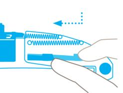
Release the blade carrier by **pressing down** and pushing forward, as indicated.
