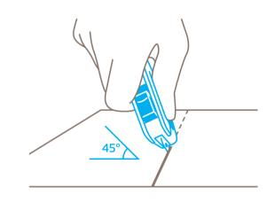
For best results, hold the cutter at **a slight** angle when cutting adhesive tape.
