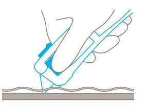
When cutting foil, be sure there is **enough counter-pressure** that the blade does not retract by itself.
