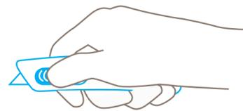
Position your **thumb** on the slider's grooved section.
